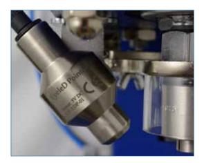
The Eyeled laser pointer assists you in the positioning of the grommets. It will be delivered with a battery case and a power pack.
