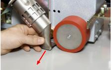
The distance from the beginning of the nozzle slot to the silicone rubber must be 3 mm.
