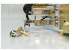
2.) Mount the seam guide onto the holder of the caster wheels.
