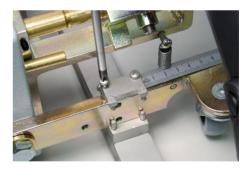
5.) By the help of tightening the backward screws of the hem guide, you can adjust the vertical and horizontal position of the hem welding kit.
