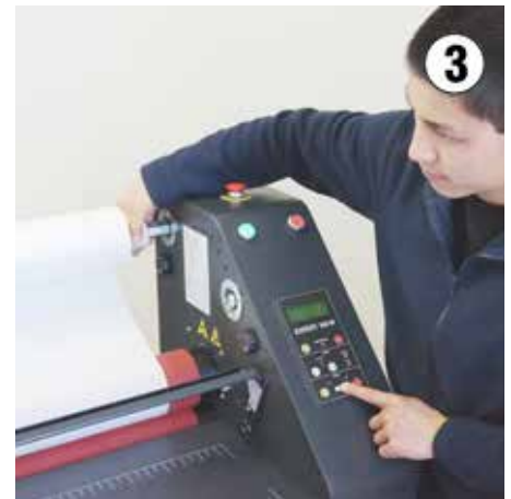
3 Wrap the laminate back tightly onto the laminate roll
