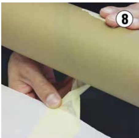
Fasten the liner to the core to wind up
