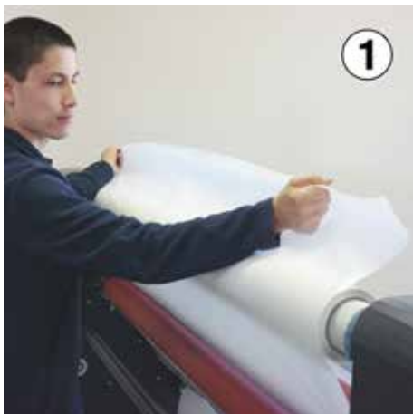
1 Lay the laminate film incl. the liner between the rollers
