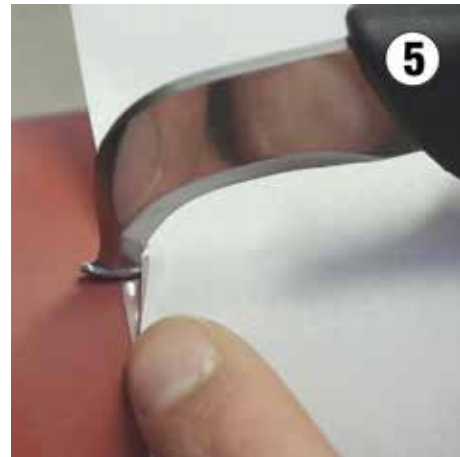
Position the blade of the EASYLAM-CUTTERs between film and liner
