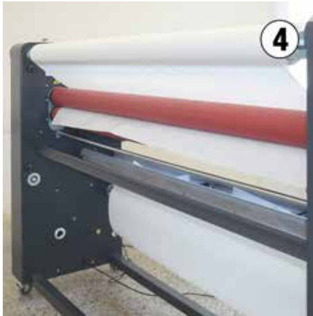
Behind the rollers of the laminator should protrude approx 5 cm
