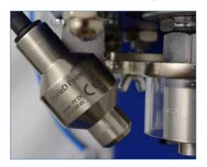
The EyeLED-pointer assists you in the positioning of the grommets. It will be delivered with a battery case and a power pack.
