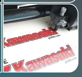
Cut huge graphics, multiple copies and perfect pin stripes without babysitting your cutting plotter. SummaCut-R's built-in media rollers and titanium coated, precision edged, media drive drum deliver vinyl through the cutter in
