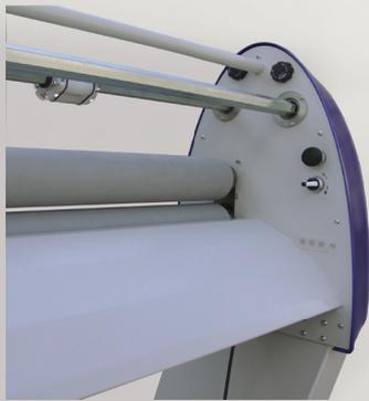
The **EASYLAM-160C CLASSICO-Line** is a large format cold laminator. Some parts of the construction are similar to the EMBLEM Avantgarde. The stand of the laminator has the same design like the MediaTrim MT 230m - the „CLASSICO-line“. The stand is optional - also the third axis. Processing versatility of 1640 mm and best technical components makes this EASYLAM 160C a professional lamination machine for mounting, sealing and both-side lamination process.
