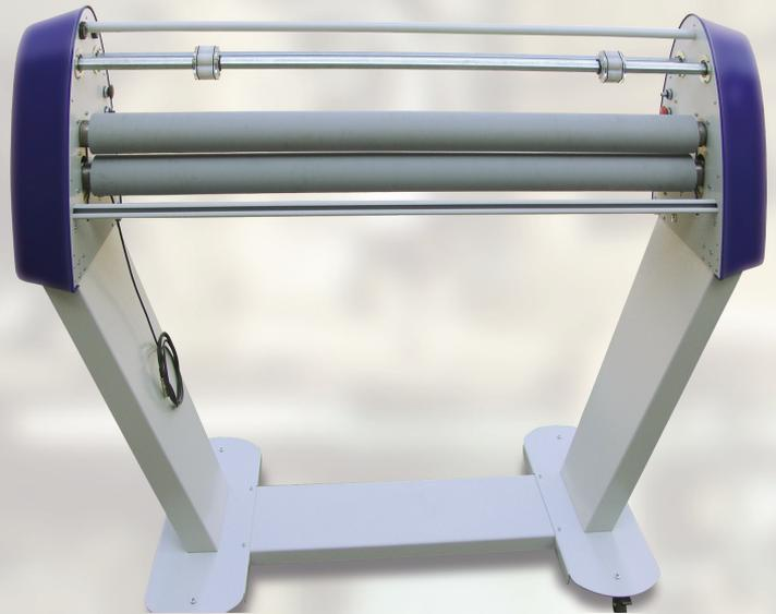
To open and close the roller is done by electrical drive and controlled by a illuminating diode. A special sensor is protecting EASYLAM 160C against over pressure and damage.
