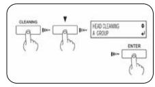
Press the [Cleaning] key, and press the [▼] key to select the printing head group to clean.
