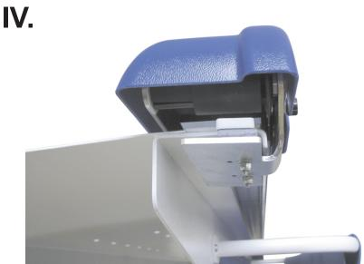
Put on of cutting head: Be carefully to both circle knife insert before flat knife.
