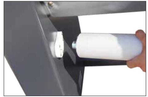
insert this end of the scroller into the left connection
