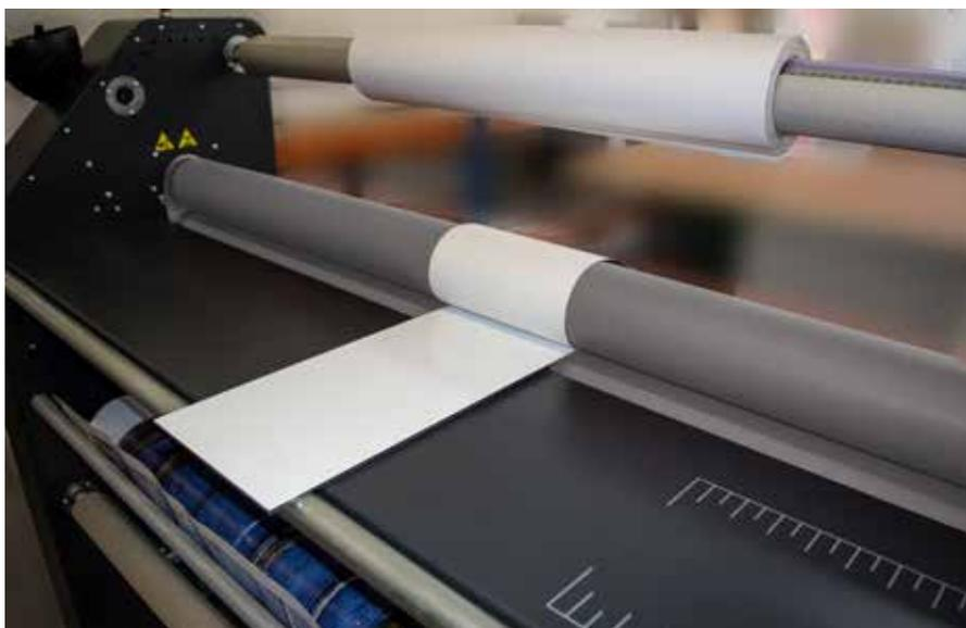
Cut the liner of one half of the self adhesive media and mount this half by using the laminator pushing “start” key.
