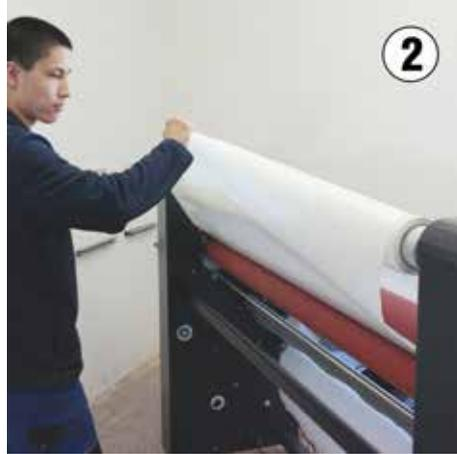
Make sure the lamination film is rolled tight
