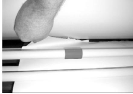
Grab the silicone paper at the bent corners and pull off for approx. 20 cm, then fix the paper by means of the 2 plastic fasteners.
