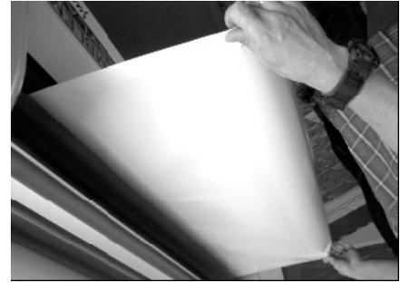
Open pressure rolls, by moving the control lever up Pull laminating film through the pressure rolls ( see below) and reset the lever in fix position.
