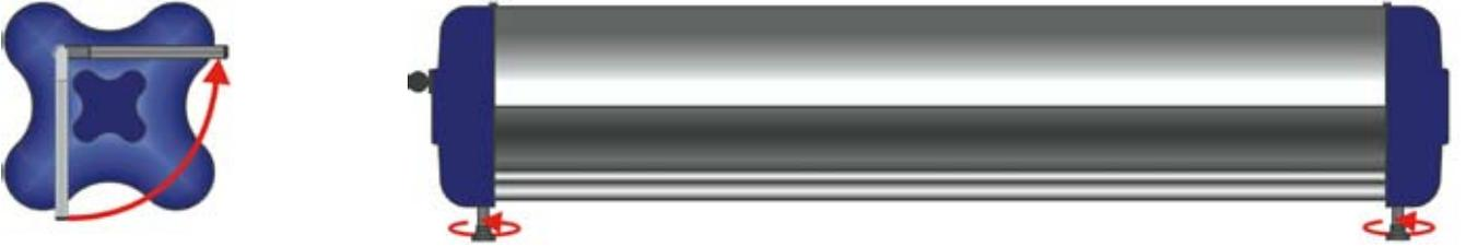
Both adjusting screws unscrew to upper stop position (position 0) in counterclockwise rotation.
