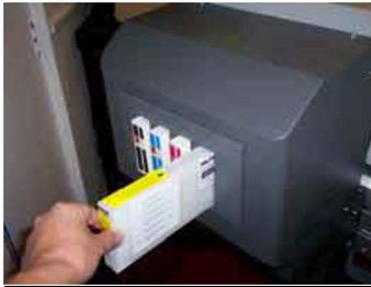
Next, remove each Mutoh cartridge one by one replacing with the EMBLEM„optimizer“ inkset, taking care that the colour removed is replaced with the identical colour from the Dataplot inkset.
