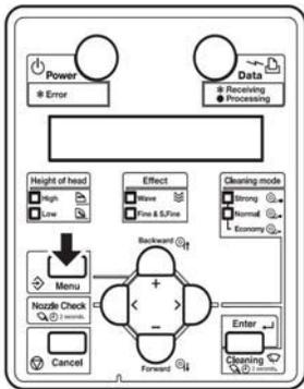
Press the [Menu] key, and press the [-] key to scroll down to *Menu4: Cleaning*, press the [>] to enter the cleaning sub menu: here you can scroll though *Economy, Normal, Strong cleans* and *Little Ink Charge*. When you find the function you require press the *Enter* key. To return to the main menu once completed press the *Cancel* key.
