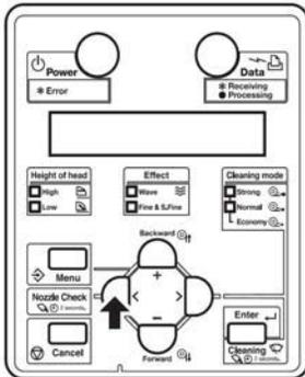
Press and hold the [**<**] key on the operation panel for two seconds or more. The printer will now perform a nozzle test.
