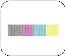
Before commencing with the ink conversion it is essential you obtain a good nozzle check (procedure for performing nozzle check is in appendix 1.) Afterwards print a setup-list directly behind it (see user's guide). No warranty dispute, regarding the conversion can be supported or defended if a pre nozzle check and a setup-list is not supplied.
